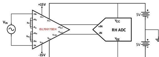
The output stage has rail-to-rail output drive capability optimized for ADC driver applications. The output stage is powered by separate supplies. This feature enables the output to be driven by the same low voltage supplies powering the ADC, thereby providing protection from high voltage signals and low voltage digital circuits. Its versatility makes it suitable for a variety of general purpose applications.
